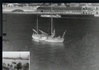
Thermal Camera with Day Picture-in-Picture
